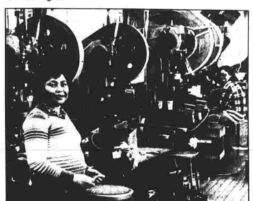
Keutn Pan-kauong is a press operator at Gunver. The presses take flat metal and bend it into various shapes later used for engine brackets.
